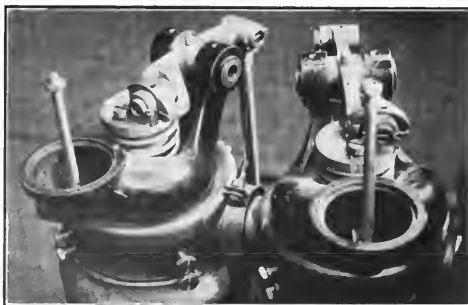
Fig. 10—Valve-operating mechanism of Panhard aviation motor
